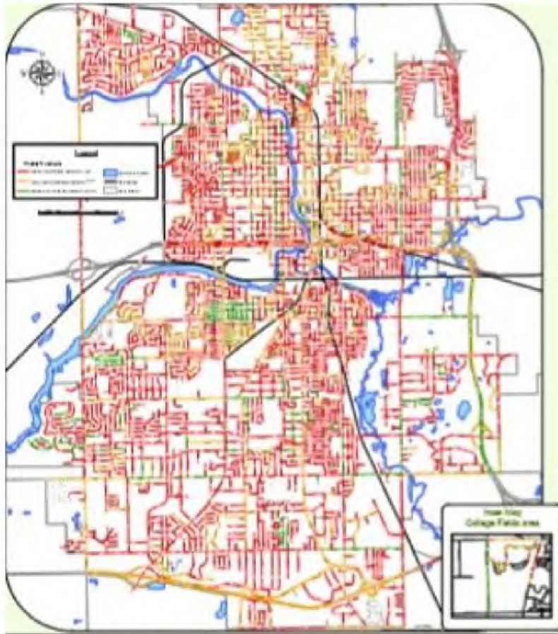
Figure 15: Map of the current paved road condition in good (PASER 10, 9, 8) shown in green, fair (PASER 7, 6, 5) shown in yellow, and poor (PASER 4, 3, 2, 1) shown in red. Only Roads owned by COL are shown.
