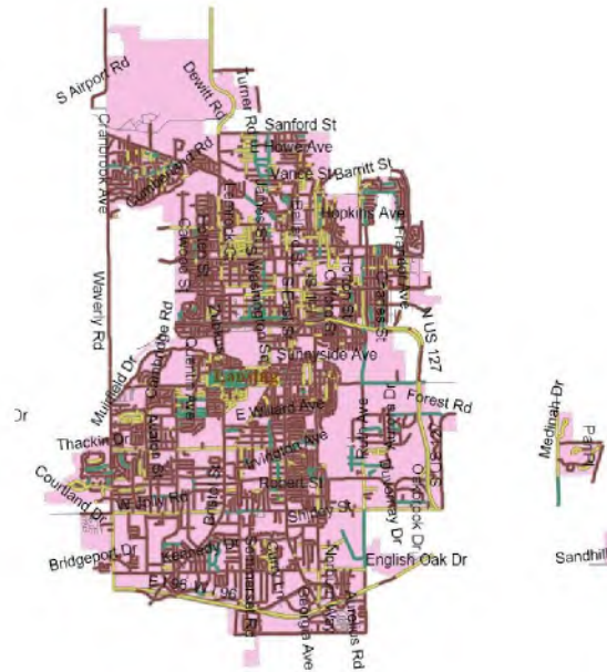
Figure 7: Map showing location of COL's paved roads (i.e., those managed by COL) and their current condition for paved roads with green for good (i.e., PASER 10, 9, 8), yellow for fair (i.e., PASER 7, 6, 5), and red for poor (i.e., PASER 4, 3, 2, 1), as well as the location of COL's unpaved roads in blue
