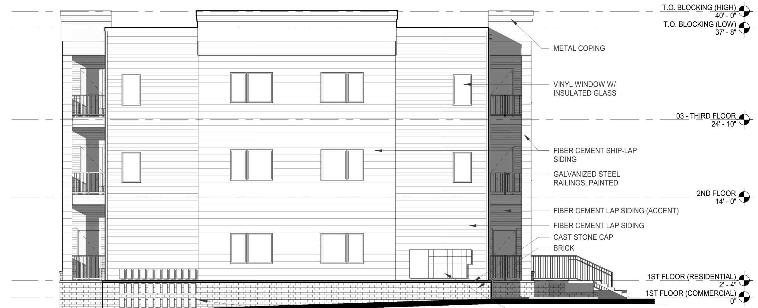
2 EAST ELEVATION (DRIVEWAY) SCALE: 1/8" = 1'-0"
