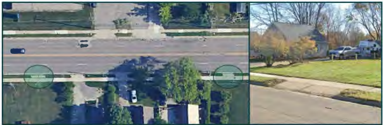
Figure 32 - Examples of unused driveway openings in the RSA corridor
