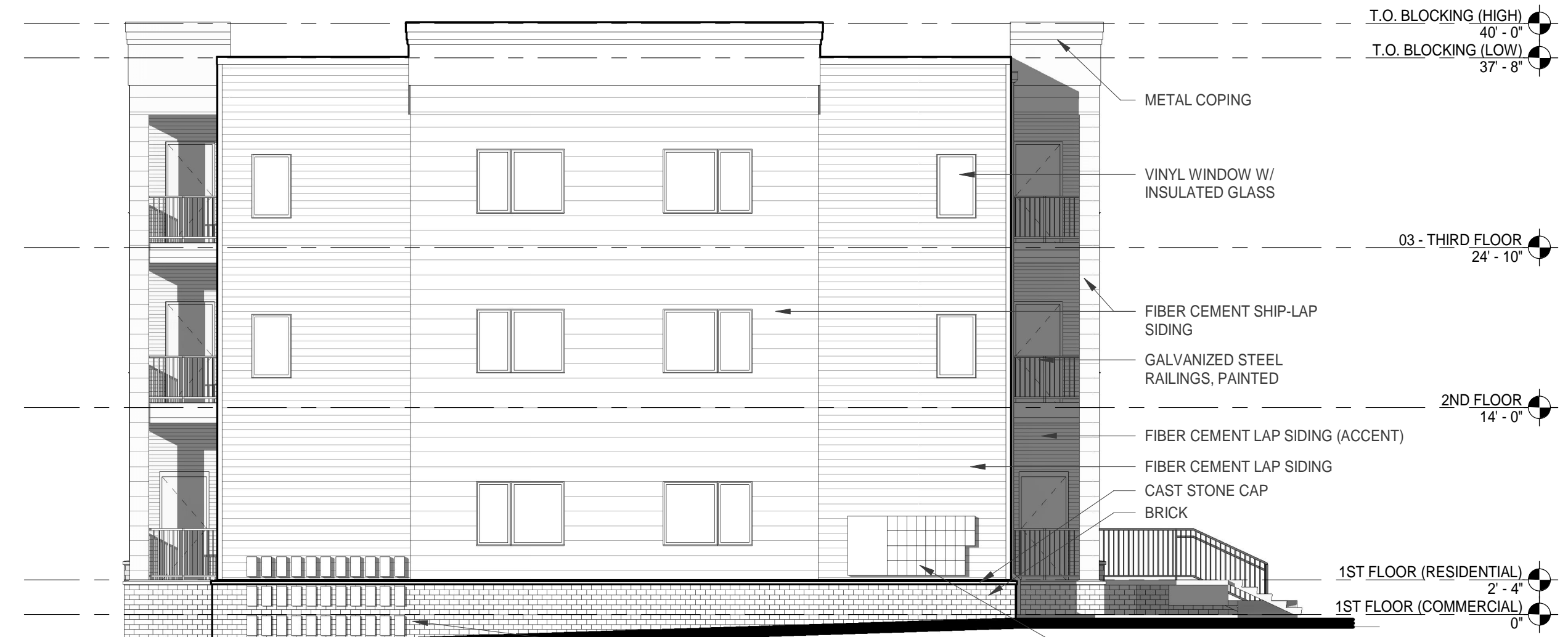
2 EAST ELEVATION (DRIVEWAY) SCALE: 1/8" = 1'-0"
